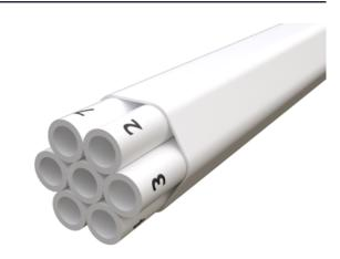
indoor installations. Every microduct has a permanent, co-extruded silicone compound inner liner giving a coefficient of friction of less than 0,1.
